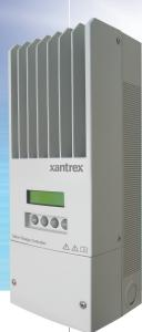
The Xantrex<sup>™</sup> XW Solar Charge Controller is a photovoltaic (PV) charge controller that tracks the electrical maximum power point of a PV array to deliver the maximum available current for charging batteries. When charging, the XW Solar Charge Controller regulates battery voltage and output current based on the amount of energy available from the PV array and state-of-charge of the battery.
